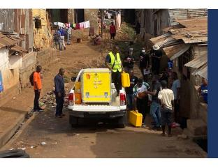
The second unit (of which one was provided) is the 'Nomad'. This is a larger system that comes in two custom built flight cases which have a combined weight of 250kg. It can be transported in the back of a pick-up truck and carried into position by the team once in closer proximity to a water source. The Nomad can produce 95 litres of safe drinking water per minute.
